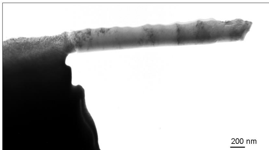
Figure 3. Bright-field TEM image of a micro beam prior to mechanical testing.
