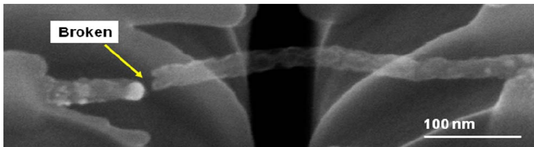
Figure 2. SEM image of a SNW after migration of the grains from the centre to the ends, transforming the SNW in carbonaceous structures.
