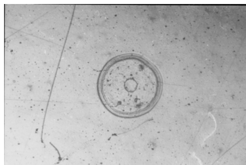
Figure 6. Magnification of one of the spots on the surface of the negative. The central circle is of an ideal shape. However, the larger circle which possibly originated from the spread of a thermal wave, due to the inhomogeneity of the negative material, does not have an ideal form.
