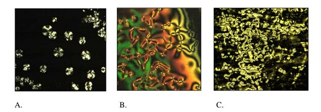
**Figure 2.** Nematic textures of the poly(butadiene)diols grafted by thiol MA with various ratio SH/double bonds in the feed (A – 0.2, B – 0.6, C – 0.8). Width of the images is about 300  $\mu$ m. The textures were observed during a cooling regime (5°C/min) at related temperatures (25°C – A and B, 72°C – C).
