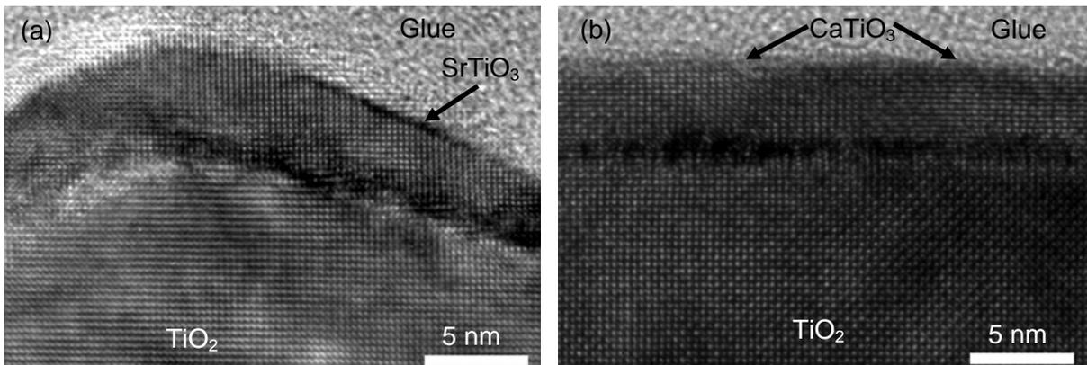
**Figure 2.** (a) HRTEM image of the SrTiO<sub>3</sub>/TiO<sub>2</sub> reaction front in [001] SrTiO<sub>3</sub>||[110] TiO<sub>2</sub> viewing direction. The sample was reacted at 700°C for ~39 min. (b) HRTEM image of the CaTiO<sub>3</sub>/TiO<sub>2</sub> reaction front in [110] CaTiO<sub>3</sub>||[001] TiO<sub>2</sub> viewing direction. The sample was made at 700°C for ~7 min.
