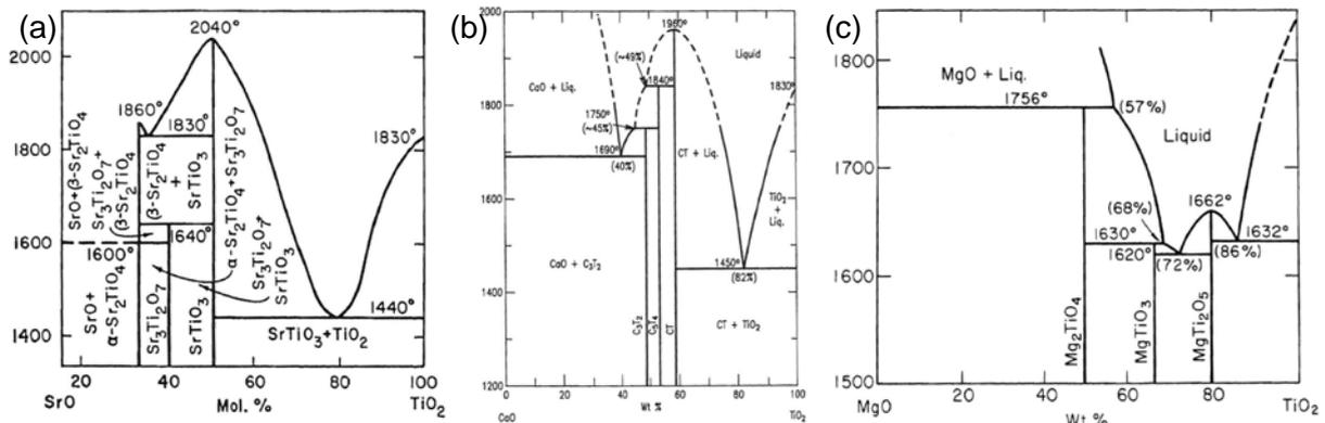
**Figure 1.** Phase diagrams of the systems: (a) SrO-TiO<sub>2</sub>, (b) CaO-TiO<sub>2</sub>. C=CaO, T=TiO<sub>2</sub> and (c) MgO-TiO<sub>2</sub>. The diagrams were taken from the book *Phase diagrams for ceramists*, ed. by M.K. Reser, American Ceramic Society, Columbus, OH, 1969.
