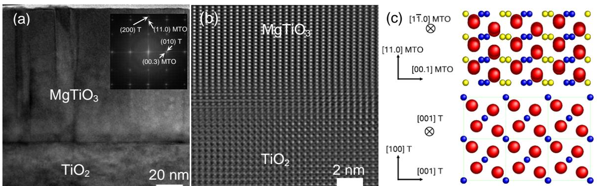
**Figure 3.** HRTEM image of the MgTiO<sub>3</sub> (MTO)/TiO<sub>2</sub> (T) reaction front. The sample was reacted at 600°C for ~35 min. The inset shows a fast Fourier transform image of Figure (a). (b) Computer-processed image of the MgTiO<sub>3</sub>/TiO<sub>2</sub> interface. Viewing direction is [110] MgTiO<sub>3</sub>||[001] TiO<sub>2</sub>. (c) Schematic cross-section representation of the interface between the MgTiO<sub>3</sub> phase and TiO<sub>2</sub> (rutile) substrate.
