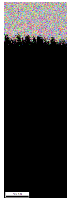
Figure 2: ChI-scan results of a CdTe thin film solar cell sample. Based on the combination of EBSD and EDS data a clear differentiation of the individual layers is possible. The maps provide microstructural information about the various films, e.g. grain size and orientation.
