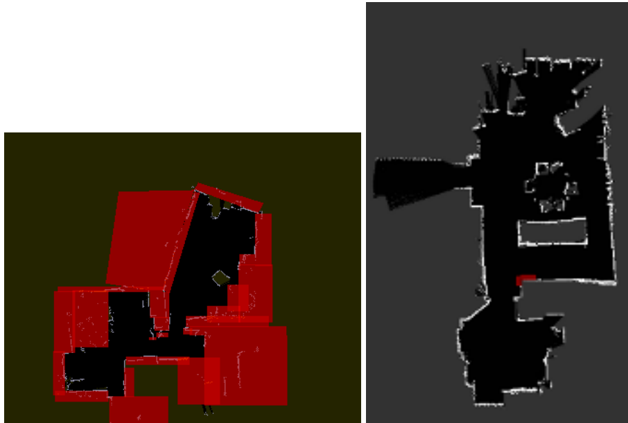
Figure 6. MIRA nogo areas can be used to avoid getting too close to corners and door sides. Note that good enough localization in the transversal direction is still very important.
