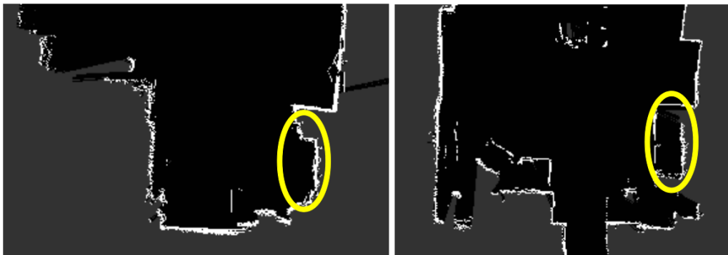
Figure 3. If the height interval considered for the bottom virtual scan is too high in the presence of low sofas, irregular borders and cushions will be present in the generated scan.
