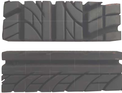
Figure 3.9.: Cut out tyre tread samples for section investigations in lateral (top) and longitudinal (bottom) direction as used on the prototype test rig
