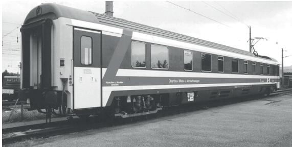
Figure 14 Standard track recording car EM250 of the Austrian Federal Railways.
