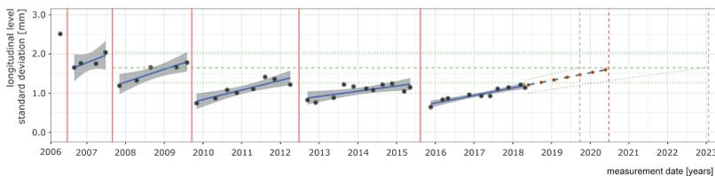
Figure 43 Principle method for predicting the next necessary tamping task.
