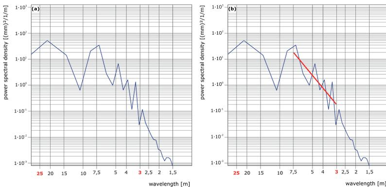
Figure 47 Power density spectrum curves based on longitudinal level measurements.
