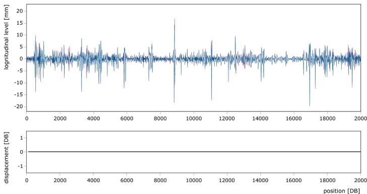
Figure 28 Validation of the post-positioning method for long track sections.
