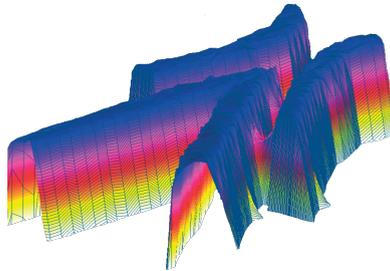
Figure 66 Common crossing wear description by using laser scan data.
