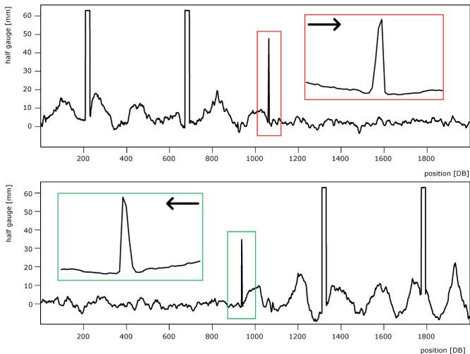
Figure 18 Half gauge signal at the common crossing for different travel directions.
