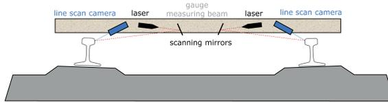
Figure 16 Working principle of the OGMS track gauge measuring system.
