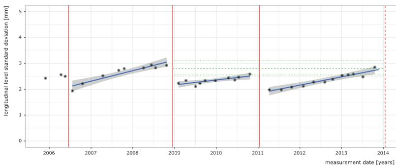
Figure 64 Tamping task prediction for the considered turnout.
