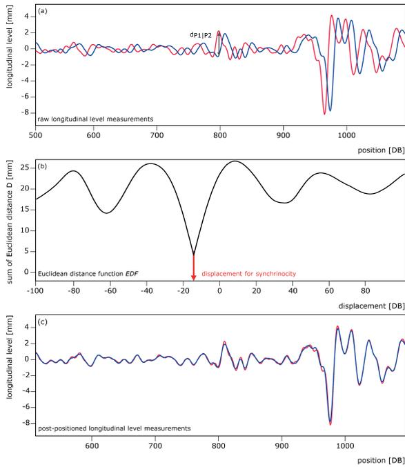
Figure 19 Principle of synchronicity validation using the EDF.
