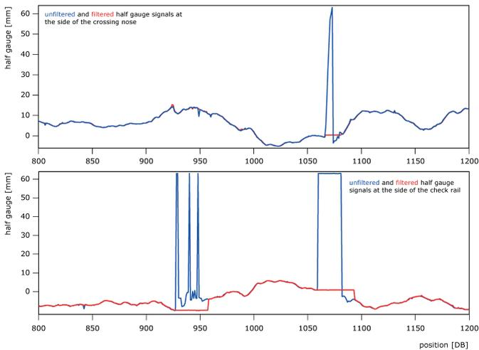
Figure 20 Synchronicity between unfiltered and filtered half gauge signals.
