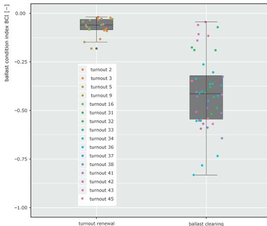
Figure 53 Ballast condition index comparison between new and cleaned ballast.
