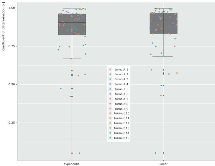
Figure 31 Comparison between linear and exponential deterioration model.
