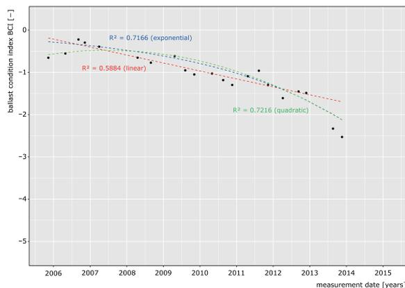
Figure 55 Adjustment of the ballast condition index deterioration models.
