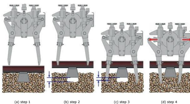
Figure 29 Basic tamping process.
