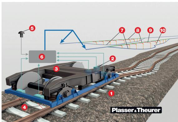
Figure 15 Working principle of the track geometry measuring system.
