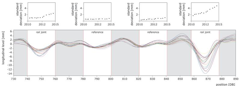
Figure 39 Analyses about the standard deviation deterioration of a jointed rail track.
