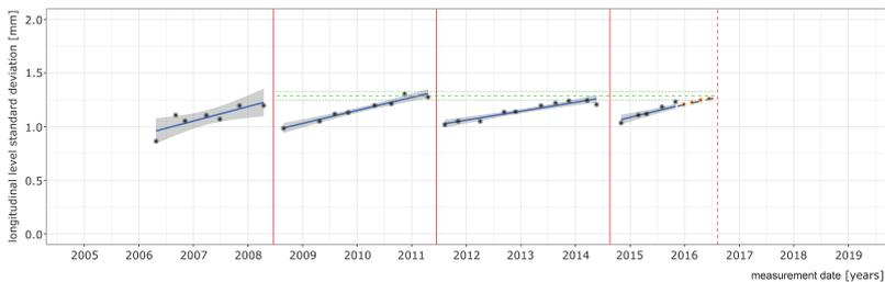
Figure 45 Predicting an additional tamping task for turnout no. 9.
