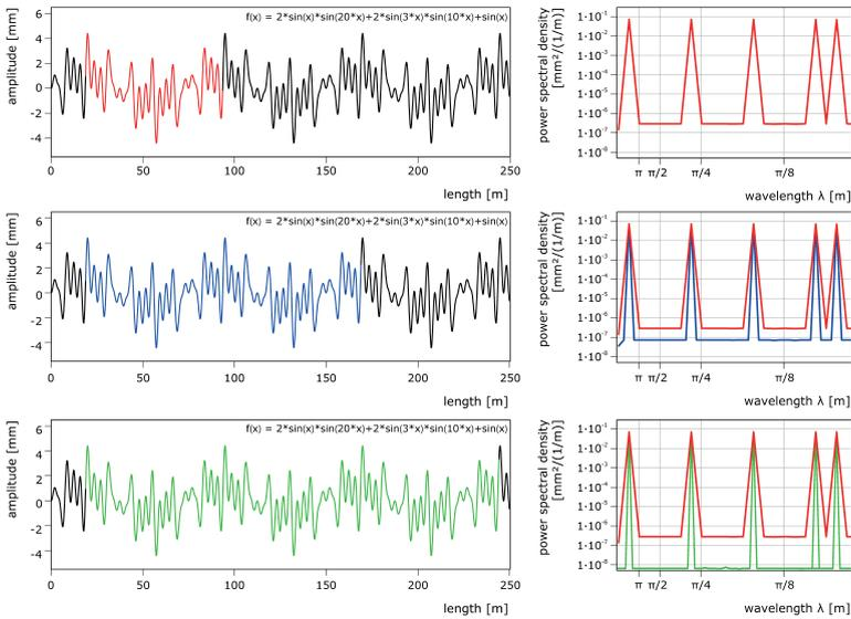
Figure 49 Result comparison of different data lengths power density calculations.
