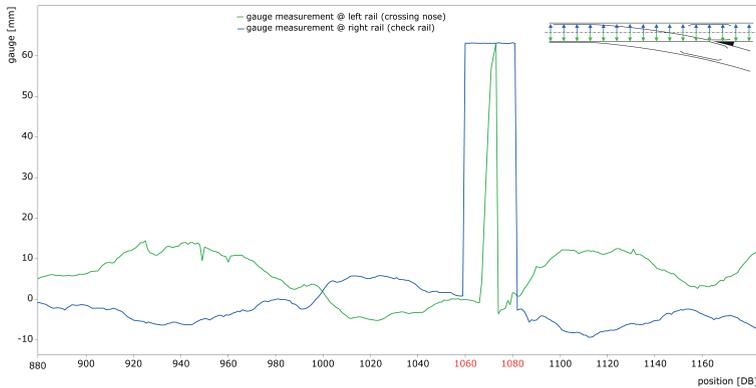
Figure 17 Half gauge measurement signals to identify a turnout.
