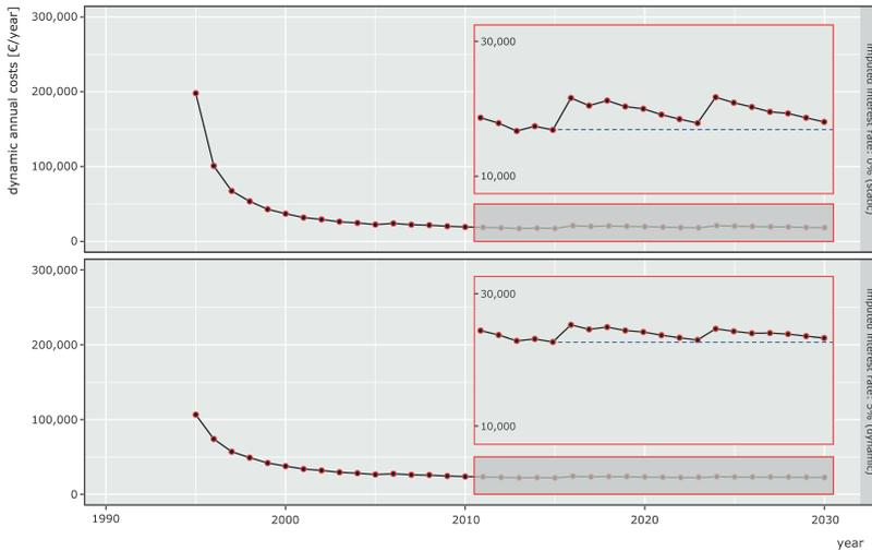
Figure 69 Annuity curve in case of a second necessary ballast cleaning in 2023.
