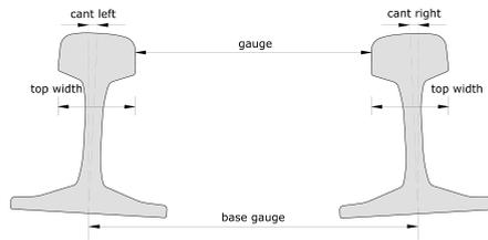
Figure 22 Different gauge measurement values.
