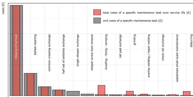
Figure 9 Comparison of unit and total costs for different maintenance activities.
