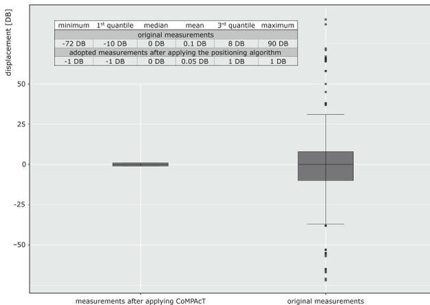
Figure 26 Example of a final control plot for post-positioned measurement signals.
