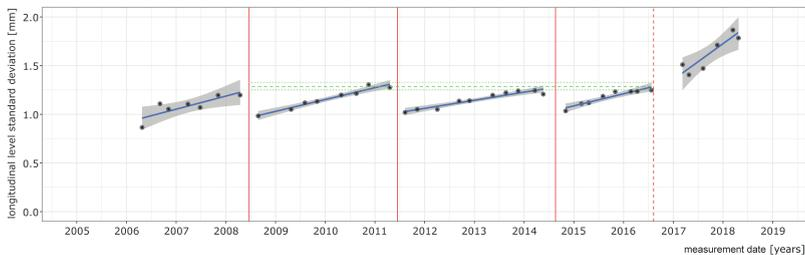
Figure 46 Comparison between the prediction and the real behaviour for turnout no. 9.
