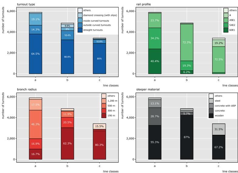
Figure 7 Superstructure and turnout geometries for different line classes in Austria.
