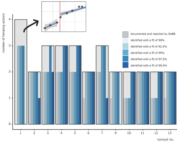
Figure 34 Identified tamping actions as a function of the prediction interval width.
