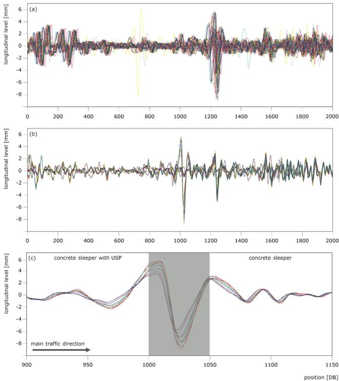
Figure 27 Example analyses to show the migration of a single failure - TwinPEAKs.
