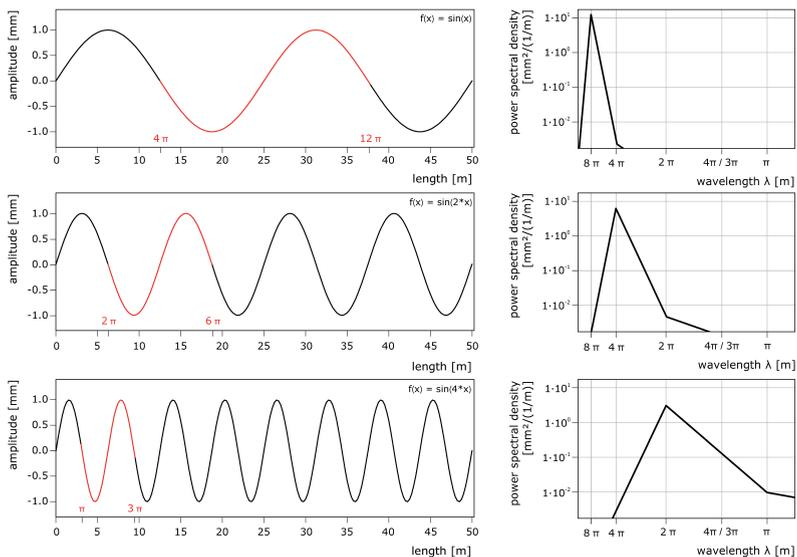
Figure 48 Results of power density calculations for different input signals.
