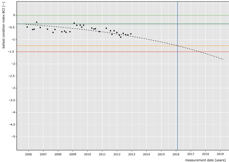
Figure 63 Ballast cleaning prediction for the considered turnout.
