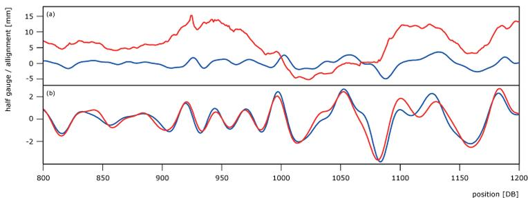
Figure 23 Relationship between half gauge and alignment measurements.
