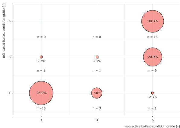
Figure 54 Comparison of subjective and data-based ballast condition grade.
