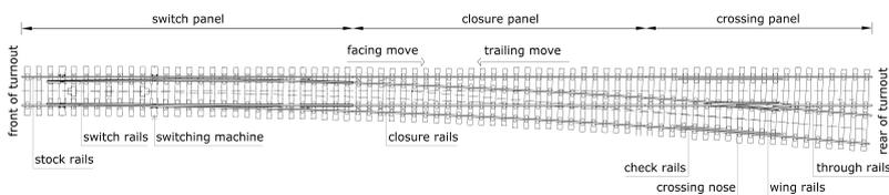
Figure 5 Designation of different turnout components.
