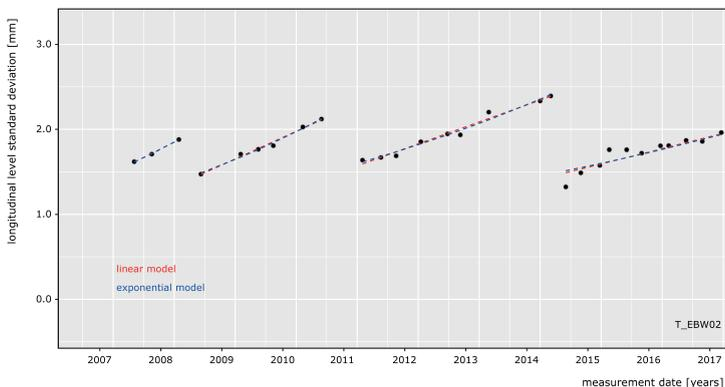
Figure 30 Linear and exponential standard deviation deterioration trend.
