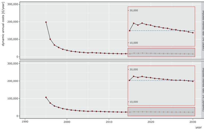
Figure 70 Sensitivity analysis about the tamping interval after ballast cleaning.
