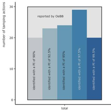
Figure 35 Results about the investigations according to the prediction interval width.
