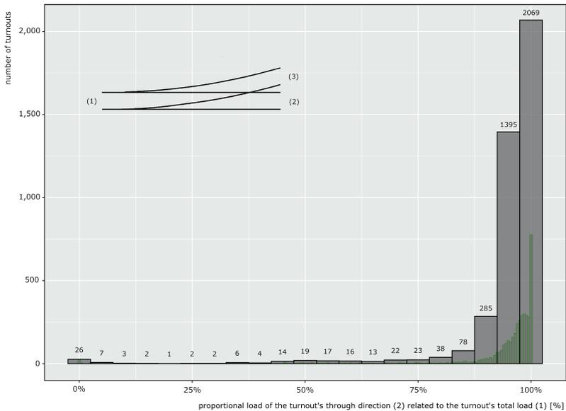
Figure 13 Proportional load of the turnout's through direction.
