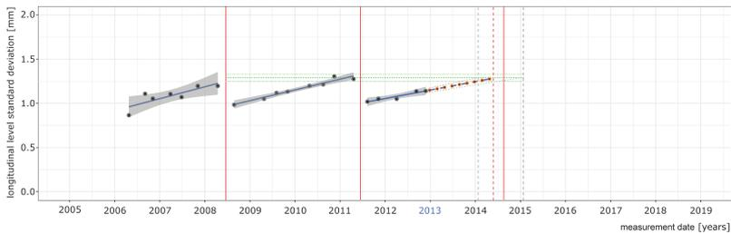
Figure 44 Predicting the next tamping task for turnout no. 9.
