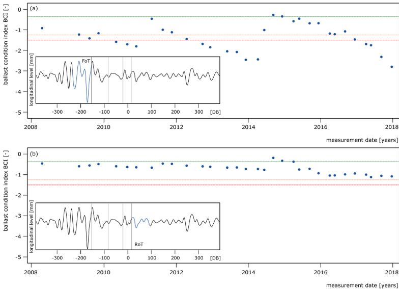
Figure 60 Ballast condition development before and after the turnout.
