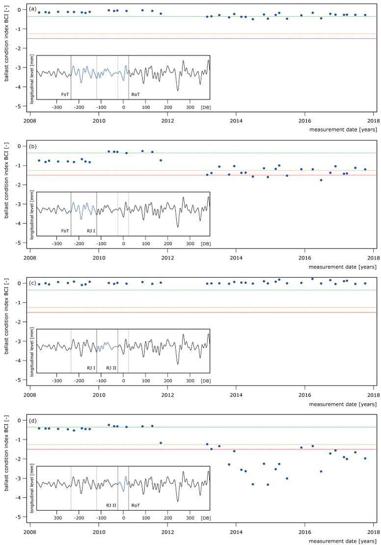
Figure 59 Ballast condition development for different turnout areas.
