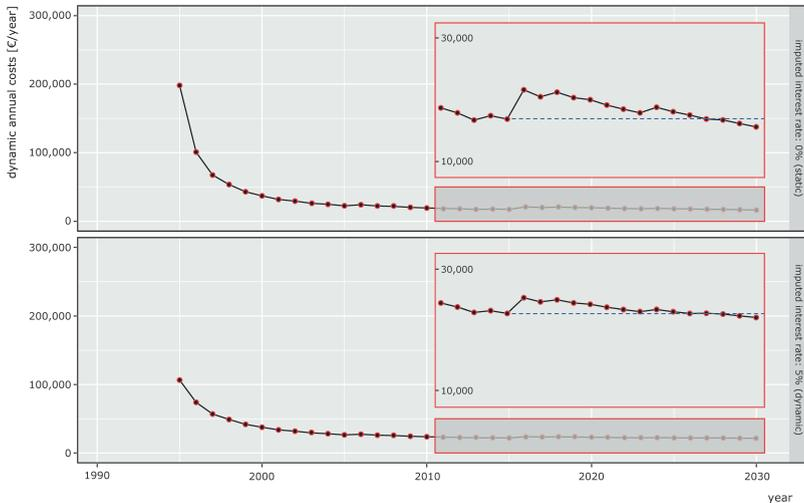
Figure 71 Annuity curve for a second common crossing exchange in 2024.
