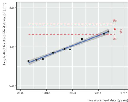
Figure 33 Case distinction to compare prediction and measured value.
