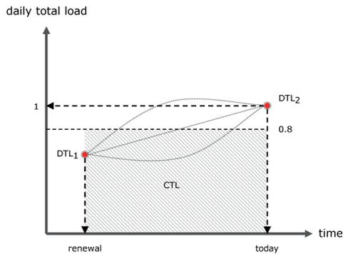
Figure 57 Cumulative total load calculation model.
