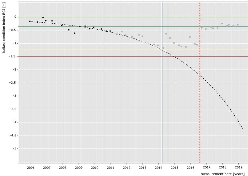
Figure 61 Model based prediction of a ballast cleaning task.
