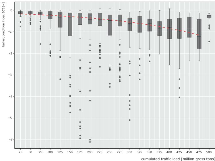
Figure 58 Summarised ballast condition index development over the cumulated load.
