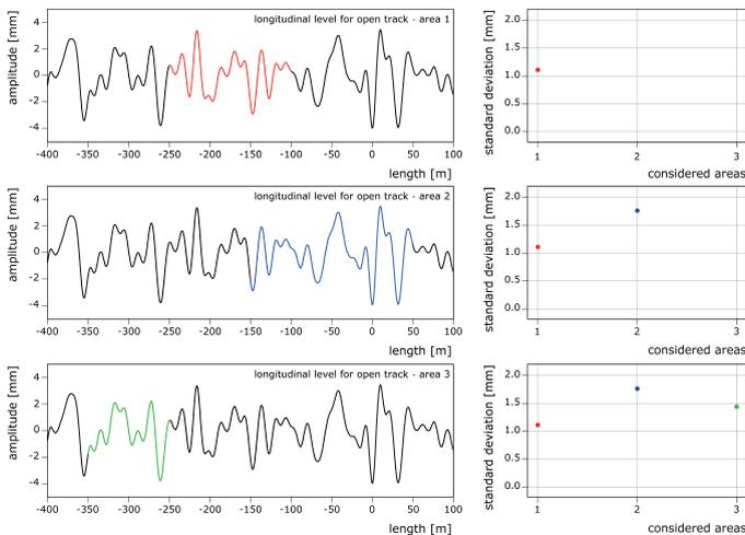
Figure 37 Influence of input data length on the longitudinal level standard deviation.
