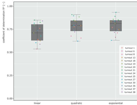
Figure 56 Comparison of different BCI deterioration models.
