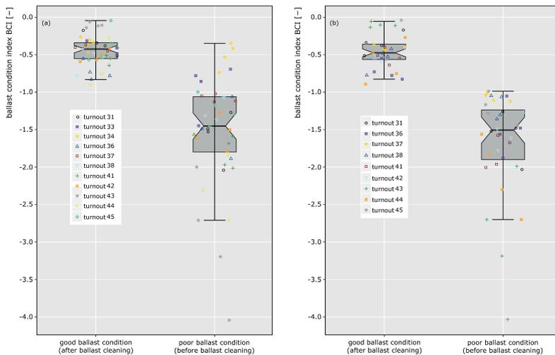
Figure 51 Ballast condition index before and after ballast cleaning.
