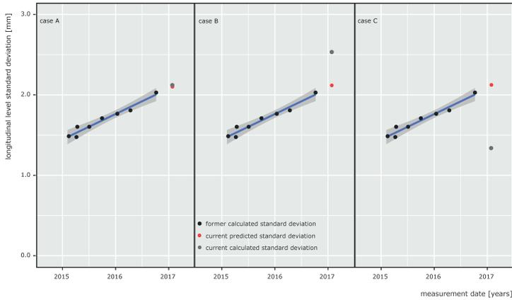
Figure 32 Case distinction to compare prediction and measured value.
