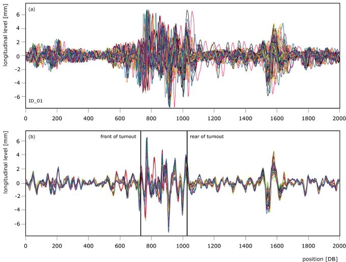
Figure 25 Longitudinal level signals before (a) and after (b) post-positioning.
