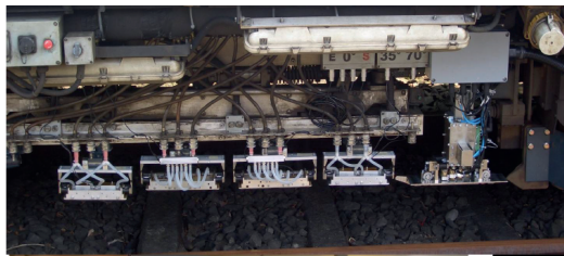
Figure 86: Ultrasonic measuring device on a measuring train [155].
