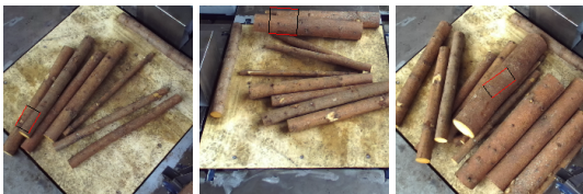
Figure 8. Examples for non-graspable predictions. ( Left ) predicted bounding box not graspable because another object is on top; ( middle ) box too big; ( right ) box too small.
