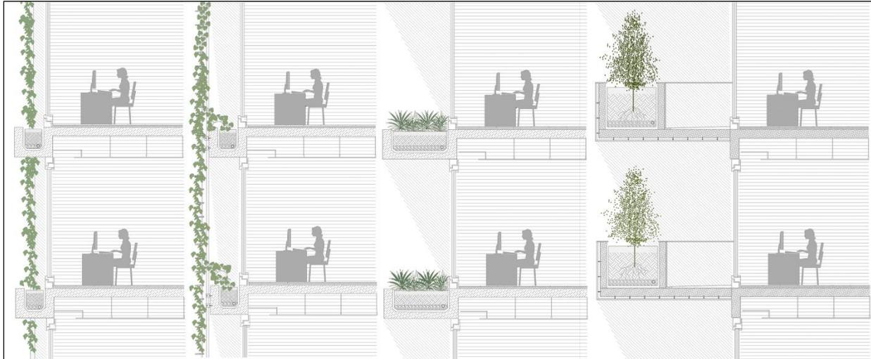
Figure 3: Simulated scenarios for different green facade design strategies;  $S_{1B}$ ,  $S_{1C}$ ,  $S_{1D}$ ,  $S_{1E}$
