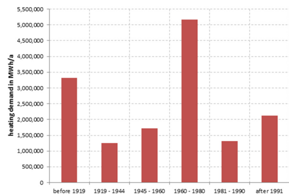
Figure 1: Total heating demand of all large-volume residential buildings per epoch according to IEE project TABULA, 2009 to 2012
