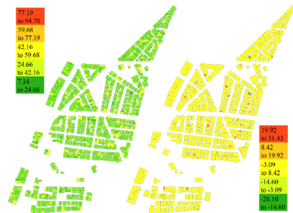
Figure 3: Izmir cooling demand (left); predicted demand error spatial distribution (right), kWh/sqm
