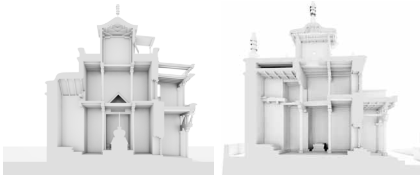
Fig. 510 The longitudinal sections of the three-storeyed Temples of Alchi (left) and Wanla (right) in Ladakh, based on the documentation in 2003 © Neuwirth & Auer, TU Graz 2020.
