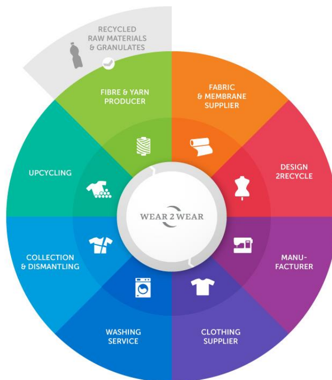
Figure 2. The wear2wear production loop. Starting from the light green field, the fibres are spun either from virgin PES or recycled granulate. The fabric is a three layered laminate just made of PES to guarantee optimal recycling at the EoL, where new fibres are made again from remolten granulate (wear2wear™, 2020).
