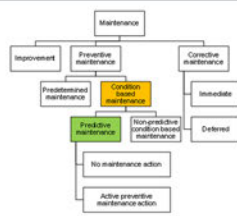
Fig. 1: Maintenance according to DIN EN 13306 [1]
