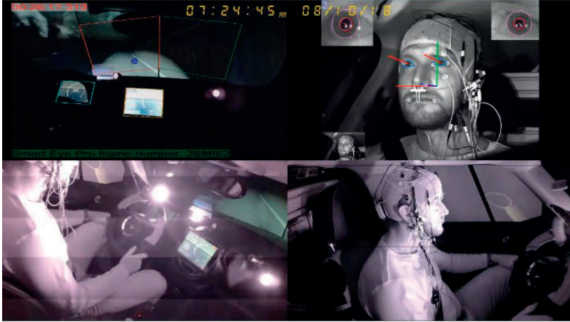
Figure 2.8: Four different views from a driver that are gathered using installed cameras inside the simulator.
