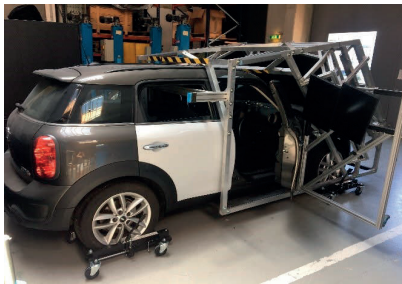
Figure 2.1: The Advanced Driving Simulator of Graz (ADSG) is a modified production car pictured here without the external housing that separates the whole simulator from the environment during the tests (left). The test track from the driver's view simulated a night drive on a highway (right).
