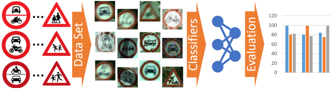
Fig. 1: Overview of the experimental setup. Starting from three sets of traffic sign pictograms (each of a different design) a large collection of embedded and corrupted images (pictogram + traffic sign + background) is created. These images are then used to train classification models. Comparing the performance of the models allows to draw conclusions about the machine readability of the initial pictograms.
