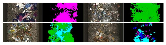
Fig. 1. Mono-material stream samples and binary segmentation belt/waste (top row) and synthetic ground-truth data with mixed stream (bottom row). All images: plastics (green), wood (turquoise), textiles (purple), paper (blue).
