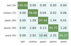
Fig. 2. Confusion matrix with pixel-wise accuracies in % for 324 test images. Apart from minor confusions between *wood* and *paper*, the performance of the CNN model is very promising.
