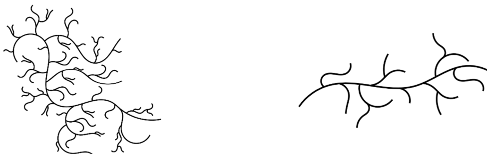
Fig. 2.: The microstructure of LDPE produced in autoclaves (lef) and tubular reactors (right). Due to the back-mixing behavior of an autoclave, its product is tree-like branched. Tubular products are comb-like branched.
