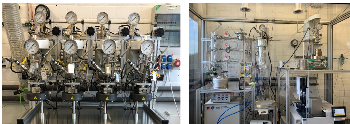
Figure 1: 4-Fold multi-batch-reactor for catalyst screening (left) and fixed-bed reactor equipped with online gas chromatograph (right).
