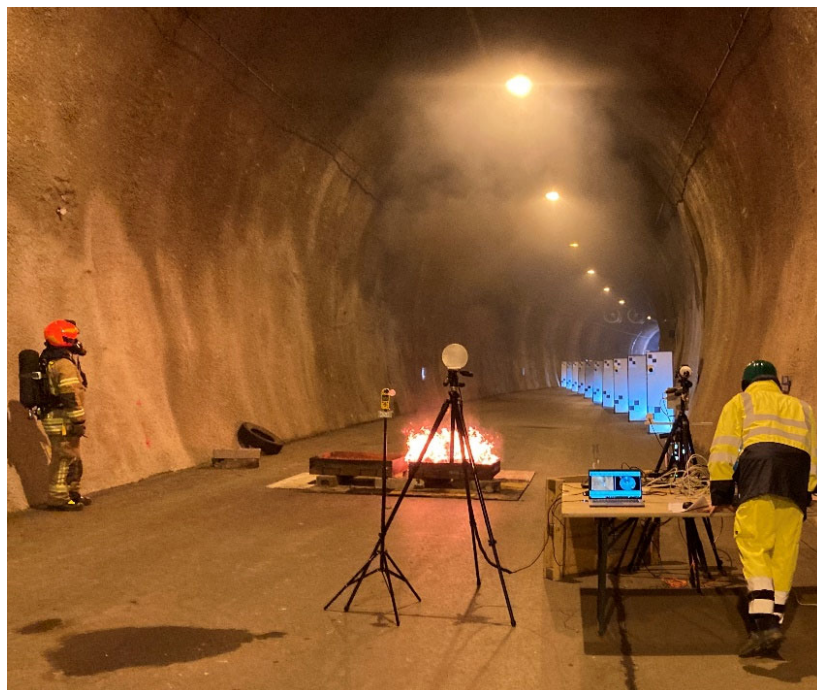
Figure 4: Fire tests for the sensor evaluation (railway tunnel, ZaB)
