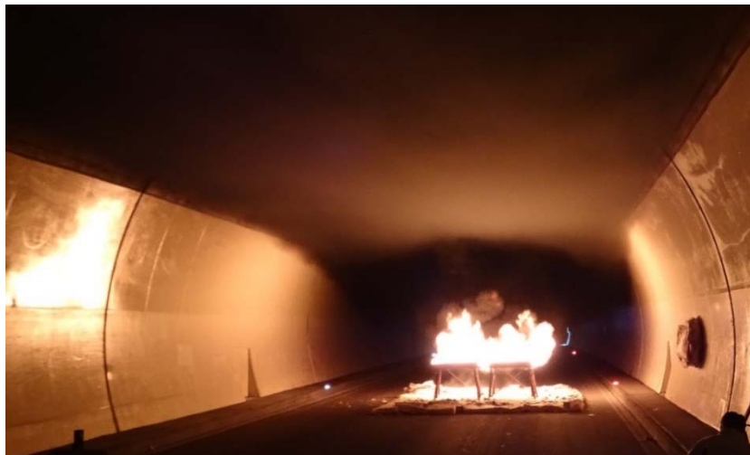
Figure 4: Smoke back-layering and downstream stratification in the first minutes of the test
