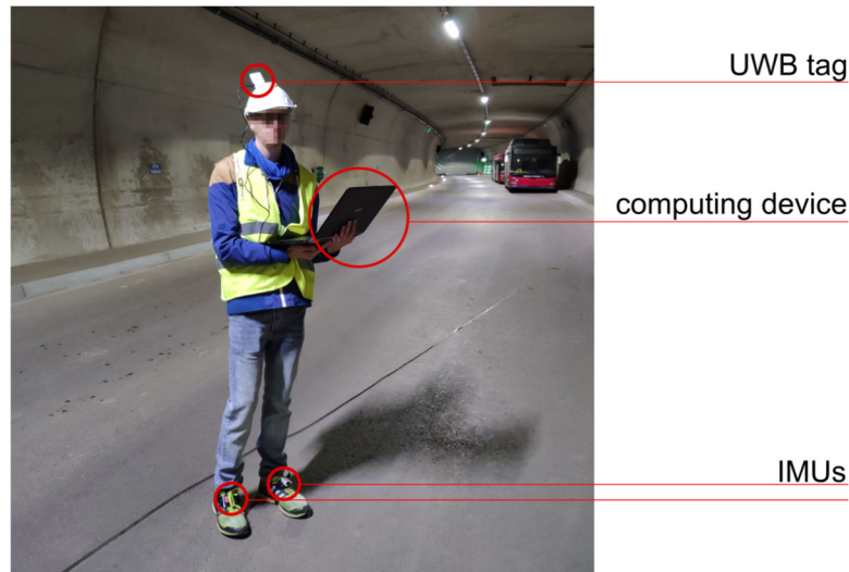
Figure 2: Test subject with sensors mounted on helmet and shoes. [1]
