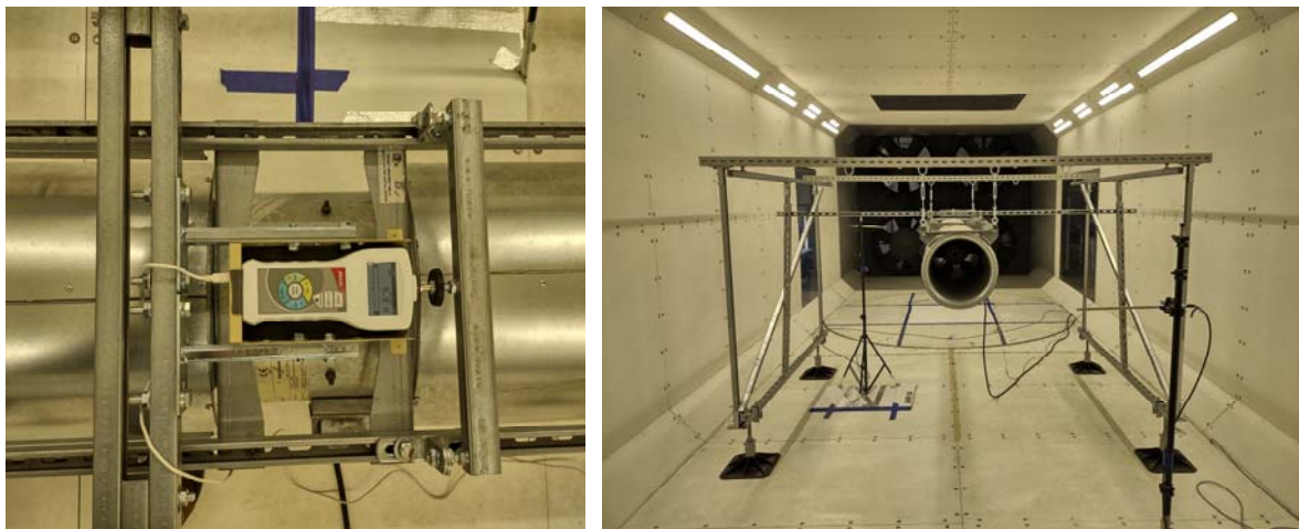
Figure 2: Thrust measurement (left) Jet Fan 355mm on the station (right)
