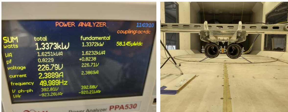
Figure 3: Power consumption measurement (left) A pair of jet fans 50mm (right)
