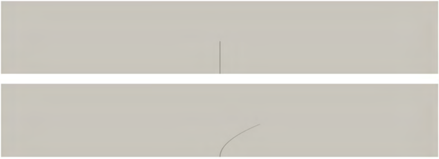
Fig. 8.23: Beam in cross-flow: fluid (light grey) and structural (dark grey) domains in initial (top) and final (bottom) configurations at t = 1 .
