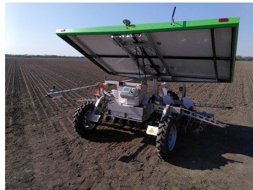
Figure 1. Field robot FarmDroid FD20 with mounted computer vision evaluation system (CVES) on the field.
