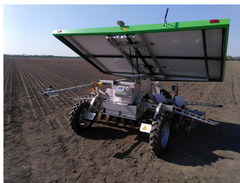
Figure 1. Field robot FarmDroid FD20 with mounted computer vision evaluation system (CVES) on the field.
