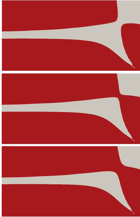
Figure 4.6: Structure optimisation: red and white areas represent high and low mass content, respectively.
