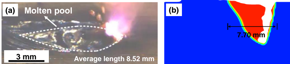
Fig. 5 Comparison between experimental and calculated molten pool length without magnetic fields: (a) experiment results; (b) calculated results (the red region in the simulation result represents the calculated weld region)
