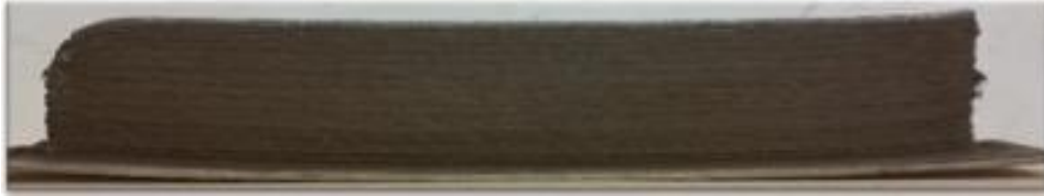
Fig. 3 WAAM fabricated 304 stainless steel plate. Note the bending of the solid base plate after release from the clamping fixtures. Lehigh University’s Additive Manufacturing Life Analysis Lab [28]
