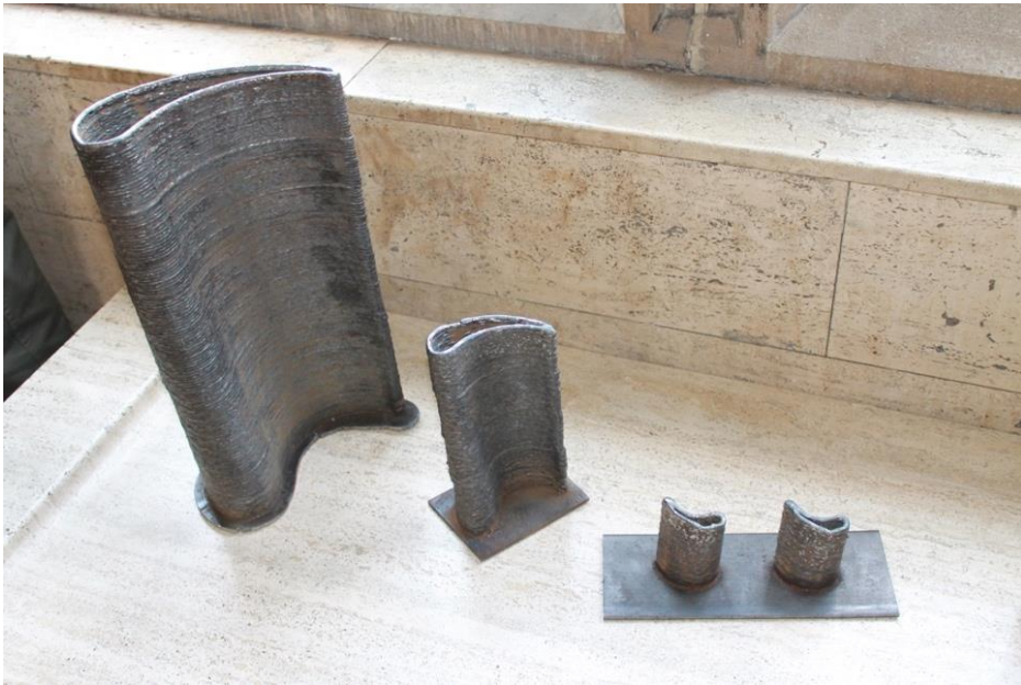
Fig. 1 Sample WAAM structural components fabricated at Lehigh University’s Additive Manufacturing Life Analysis Lab. Courtesy of Dr. C. Haden
