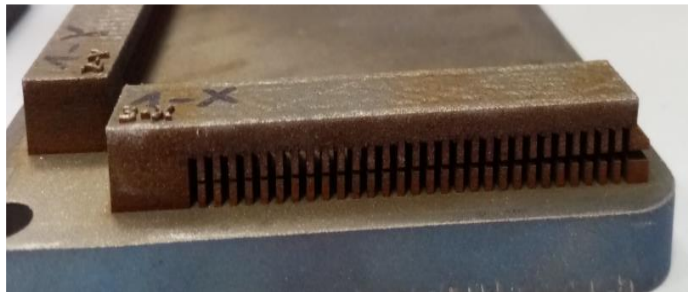
Fig. 7 Printed cantilever for experimental investigation and validation of simulation
