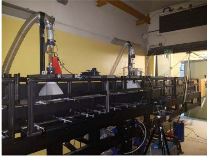
Figure 1: Picture of the experimental set up for the transverse SSD - PC ventilation system
