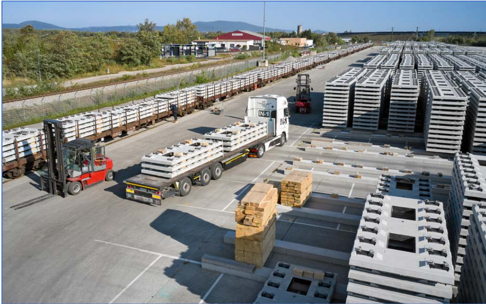
Figure 3: Track support plates transshipment from road to rail / MABA in NÖ, October 2021
