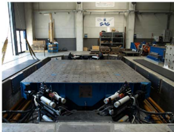
Figure 5: Multi axial shake table - courtesy of EUCENTRE [36]
