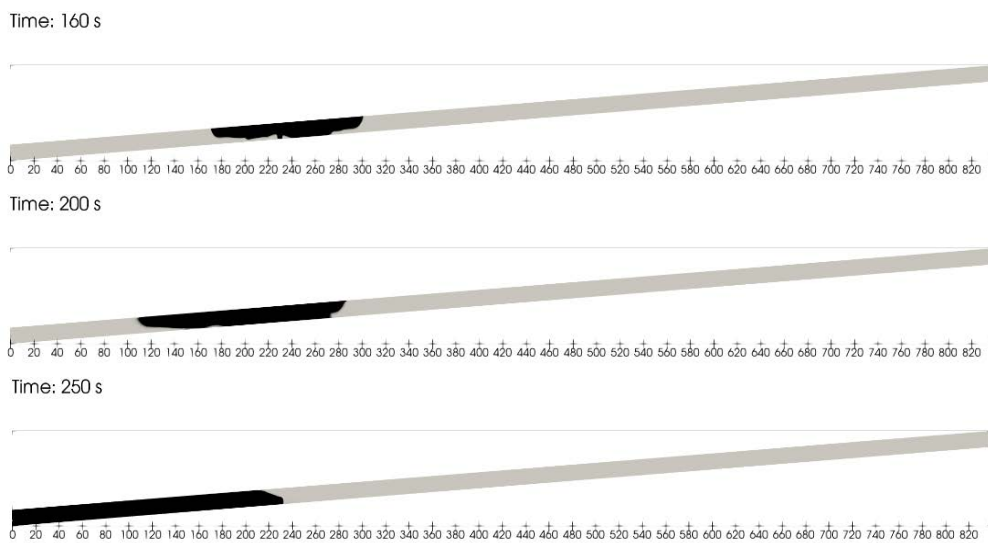
Figure 6: Smoke distribution in the Fire-eject strategy
