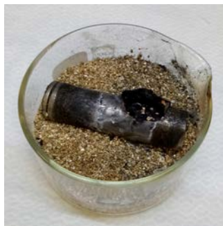
Figure 5: battery 29E after the nail penetration test.
