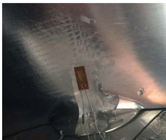
Figure 6: Strain gauge on blade
