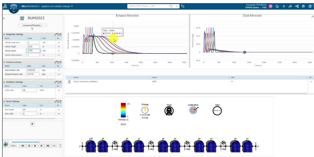
Figure 9: Web-based railway tunnel simulation dashboard on the 3DEXPERIENCE® platform.
