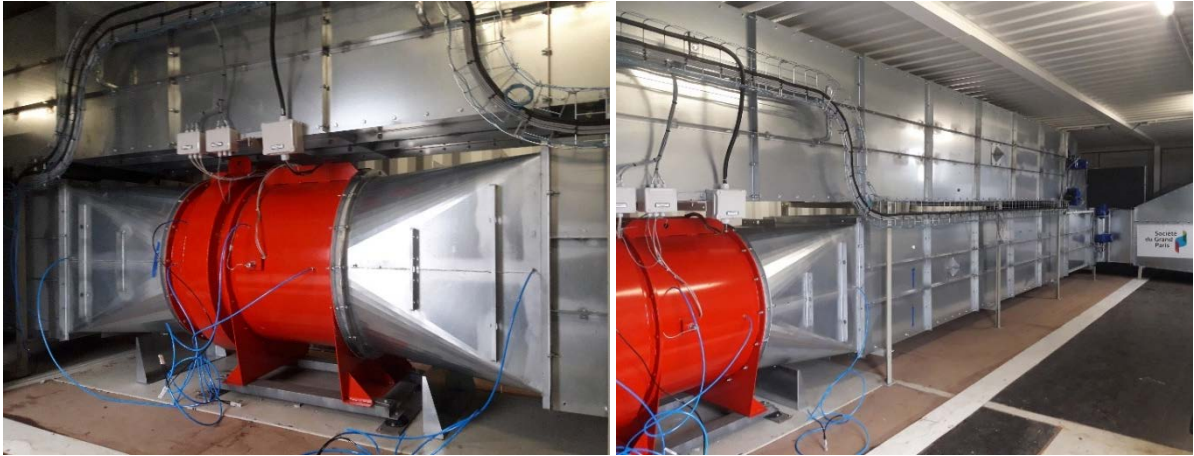
Figure 4: The model fan with anemometers and pressure probes
