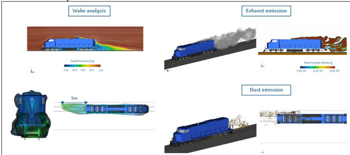
Figure 4: Advanced post-processing of 3D CFD analysis.
