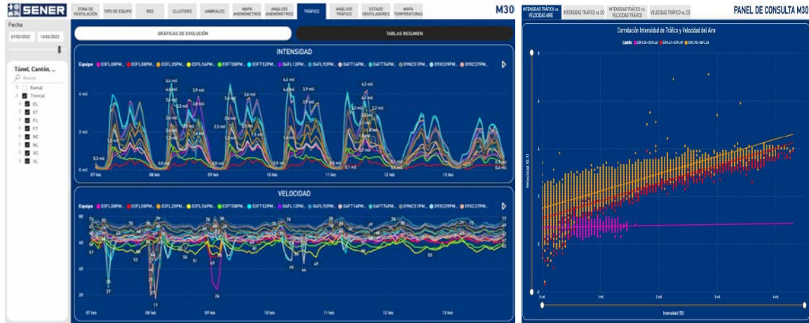
Figure 4: Correlation between traffic intensity and speed in the different areas of the tunnel.
