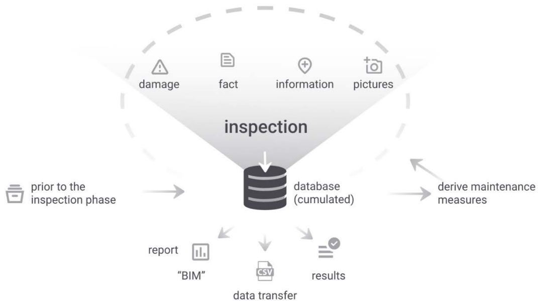
Figure 4: Schematic workflow for an inspection and documentation of inspection works and damages with emphasis on the use of a digital inspection methodology (adapted from [6])
