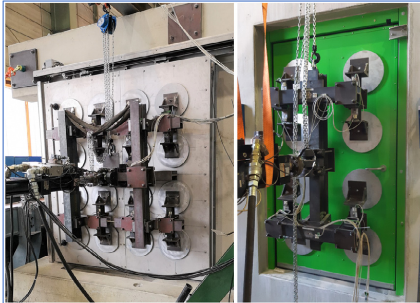
Figure 7: Emergency exit doors Koralmbahn – load tests in Vienna, March / July 2020
