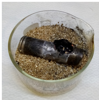
Figure 5: battery 29E after the nail penetration test.
