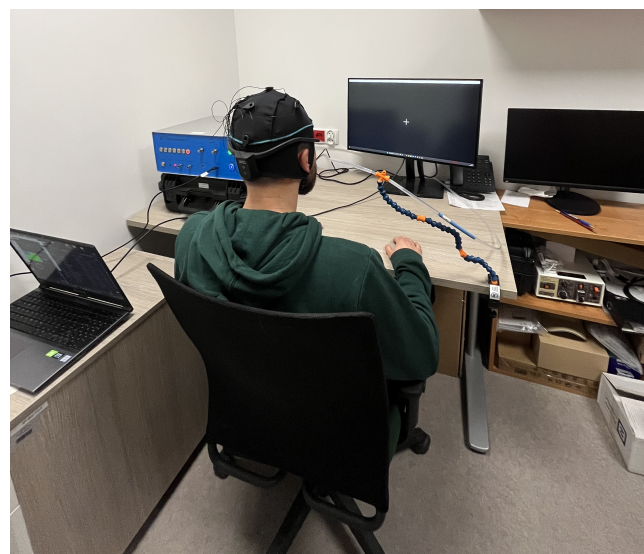
Figure 1: An experimental setting with a subject wearing an EEG cap in front of an olfactometer delivering scent stimuli.
