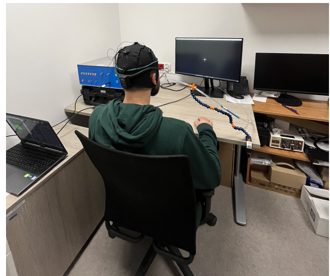
Figure 1: An experimental setting with a subject wearing an EEG cap in front of an olfactometer delivering scent stimuli.
