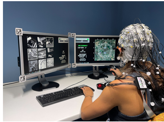
Figure 1: Experimental setup. Left Screen: Search Task. Right Screen: Navigation Task. Center Top: Flight director with task information. (Note: The text in the centre of the screens is feedback only displayed during the training phase.)
