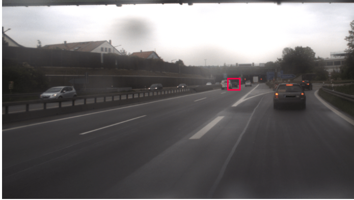
Figure 6. Example of missing ground truth label for the Rooftop dataset. The 3D bounding box of the red boxed car is missing even though it is clearly visible in the image and LiDAR data.
