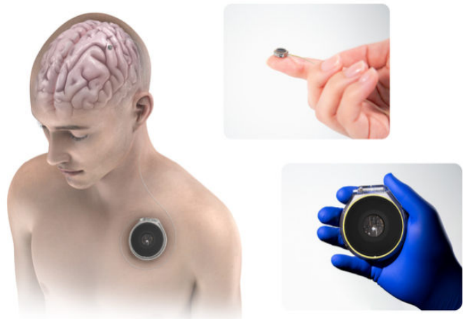
Figure 1: (Left) Rendering of the fully implanted intracranial BCI. (Right) Photographs of the Cortical Module (top) and Internal Transceiver (bottom).
