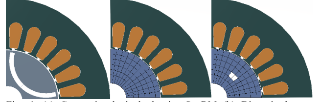
Fig. 4. (a) Conventional single barrier SynRM (b) Discretized rotor geometry (c) Controller at start position.
