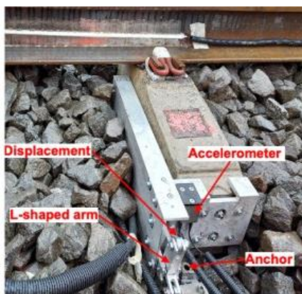
Figure 9. Detail of an instrumented sleeper equipped with a vertical base plate, an L-shaped mechanism, one accelerometer and one displacement transducer.
