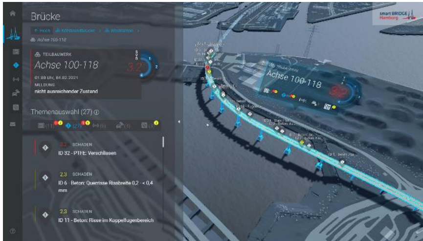
Figure 12. Visualization of structural damage information (source: MKP GmbH)
