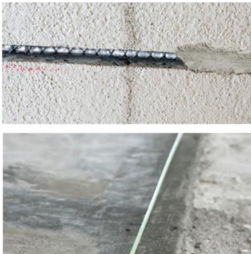
Figure 9. Installation of the EpsilonSensors with braid in near-to-surface grooves (top) and without braid directly on the concrete surface (bottom).
