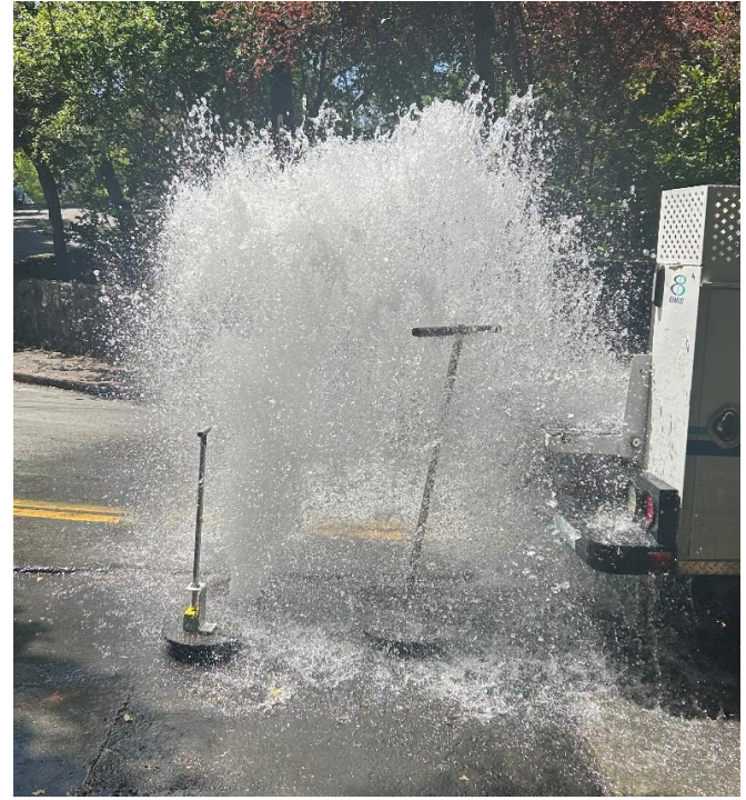
Figure 6. Simulated leakage at uphill end pipe valve
