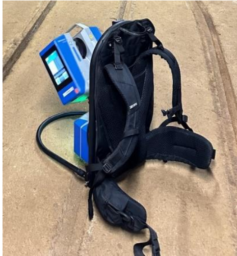
Figure 2 Z+F FlexScan22 mobile mapping SLAM platform.
