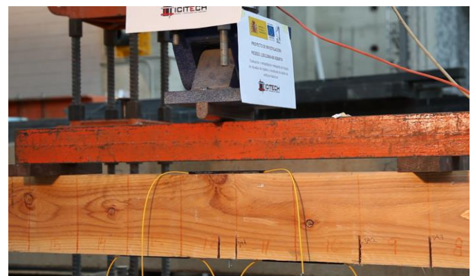
Figure 4. Central segment of the tested beam showing the loading elements.
