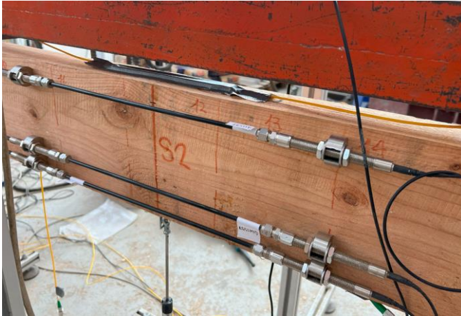
Figure 5. FOS installed in Section S2.
