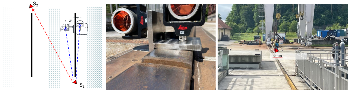
Fig. 1: The principle of measuring crane rail tracks
