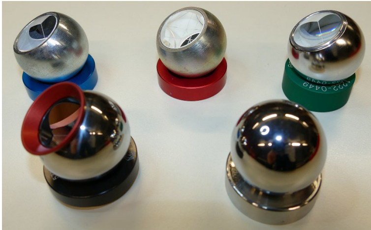
Fig. 1: Spherical glass-body reflectors of the investigated lots and higher-order references. Back: An uncertified 1445 reflector is mounted on a blue drift-nest, a certified 1445.SN reflector on a red drift-nest, and an uncertified 1448 reflector on a green drift-nest. Front: The glassless reference SMR is a red-ring reflector and mounted on a black drift-nest, while the reference steel ball is mounted on a silver drift-nest.
