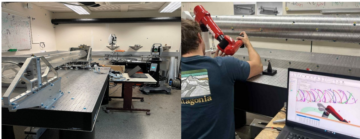
Fig. 4: Assembled deformation test bench with laser tracker (left) and groove measurement (right).
