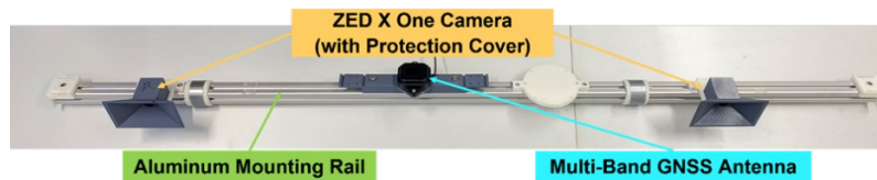
Fig. 2: System integration on the aluminum mounting rail.
