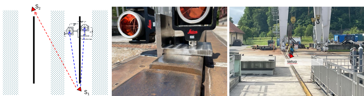
Fig. 1: The principle of measuring crane rail tracks
