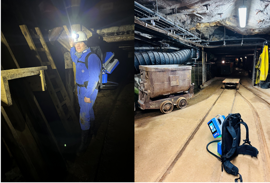
Abb. 1: Z+F FlexScan 22 mobile mapping platform with IMAGER 5016A laser scanner.
