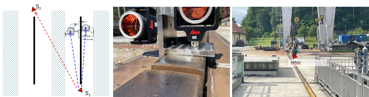
Fig. 1: The principle of measuring crane rail tracks
