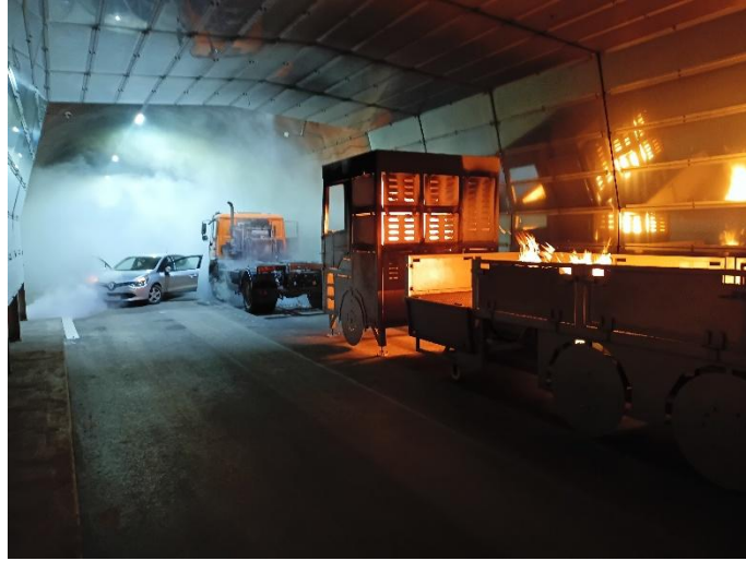
Figure 2: Truck mock-up, obstacles (cars and trucks), view opposite to direction of travel [1]
