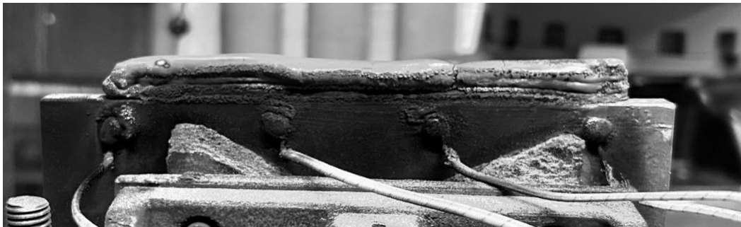
Fig. 1 Multi material DED deposition of IN718 on a CuCrZr substrate with thermocouples for temperature measurement. Bright point on the top left surface of the deposition is the laser of pyrometer.
